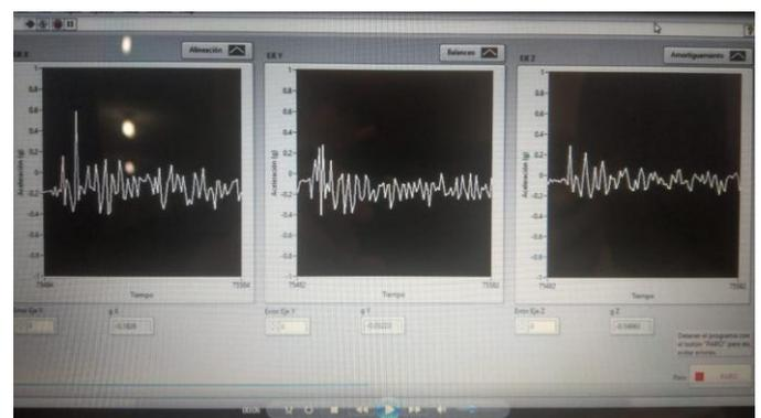
Fig -4: ADXL335 sensor result waves
