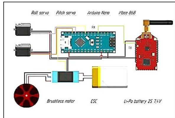
Fig-7.1: Circuit connections on the ornithopter.
