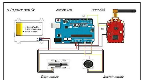
Fig-7.2: Circuit connections on the remote controller.
