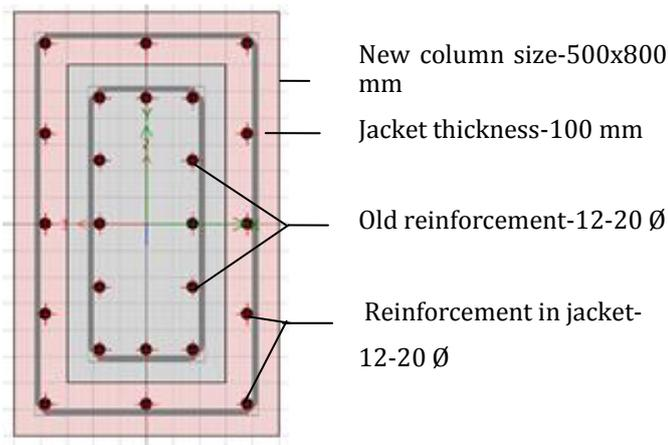
**Fig - 4:** Section of jacketed column
