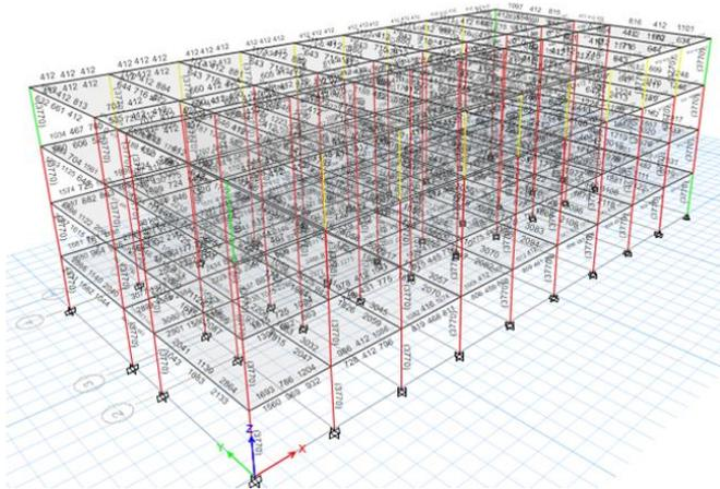
Fig – 3: Design check after response spectrum analysis
