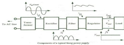
Figure Regulated power supply
