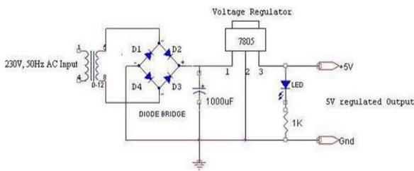
Regulated power supply is the main component of electrical, electronics and as well as automation equipment. Mobile phone charger, oscillator, amplifier are needed the regulated power supply.
