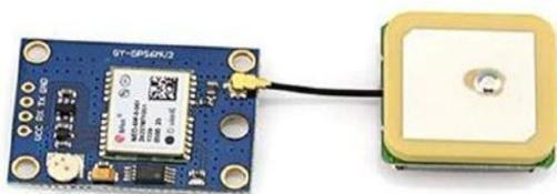
Figure NEO6M GPS Module with EEPROM, Battery & Patch Antenna
