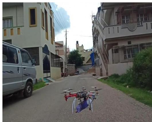
Fig 5: Hexacopter with spraying system
