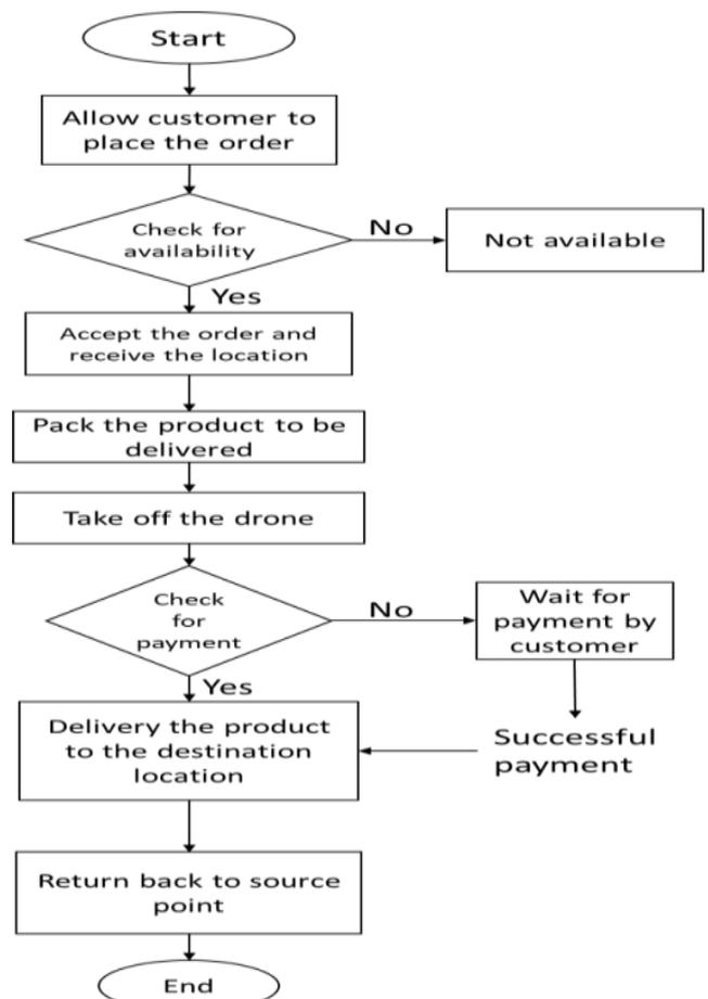
Fig 2: Flowchart of working of hexacopter
