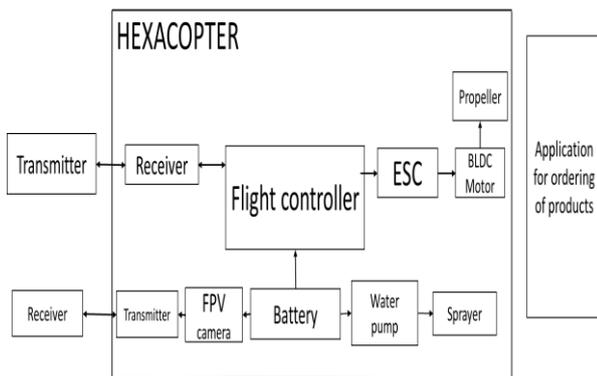
Fig 1: Block diagram of components of hexacopter
