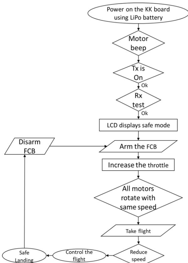
Fig 3: Flowchart of delivery system
