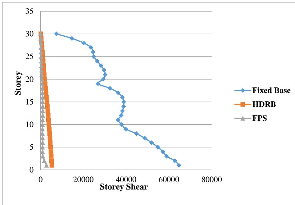
Figure 4.2.3.7: Storey Shear in X-Direction
