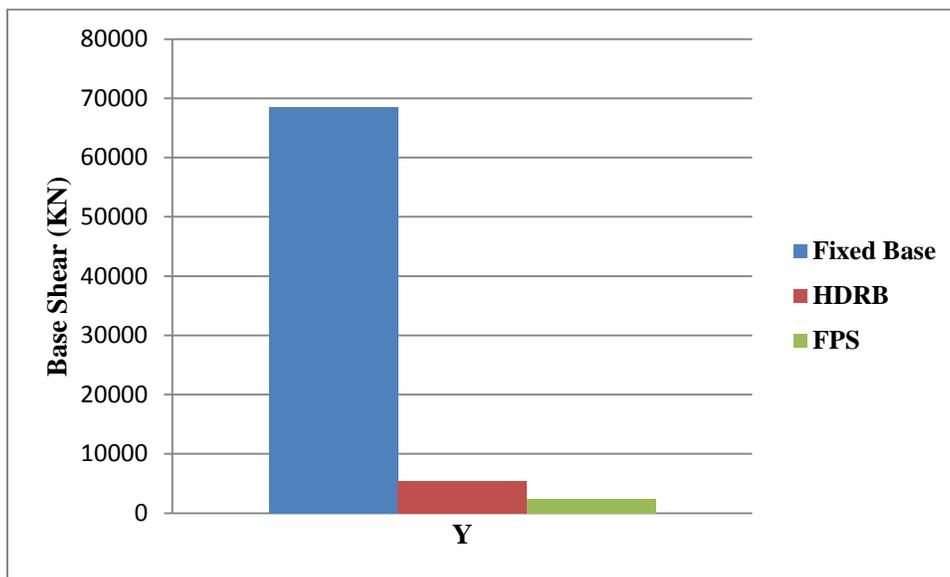
Figure 4.2.3.2 Base Shear in Y-Direction
