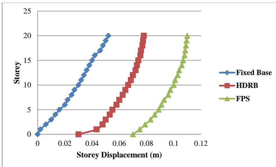
Figure 4.2.2.4: Storey Displacement in Y-Direction
