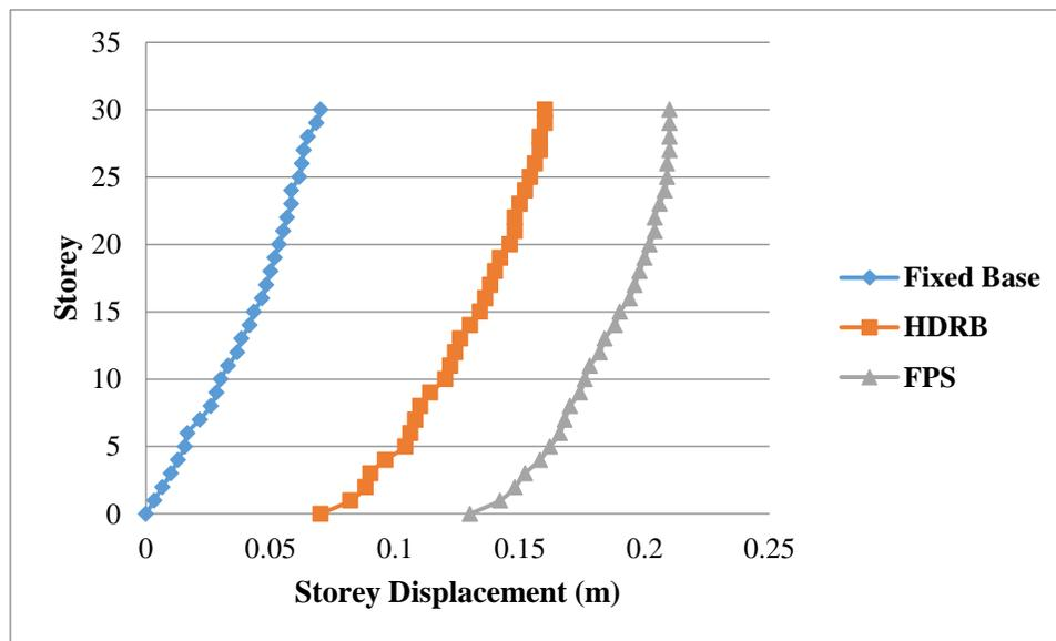
Figure 4.2.4.4: Storey Displacement in Y- Direction
