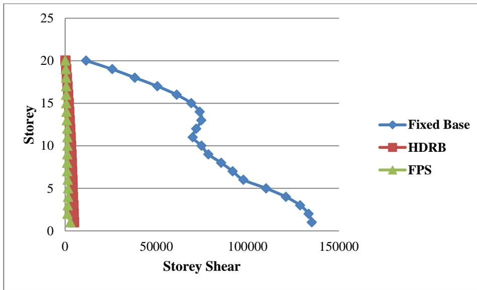
Figure 4.2.2.7: Storey Shear in X-Direction
