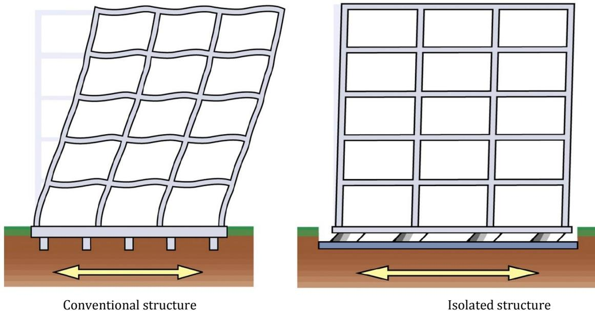
Figure 1.1.1: Behavior of Building Structure with Base
