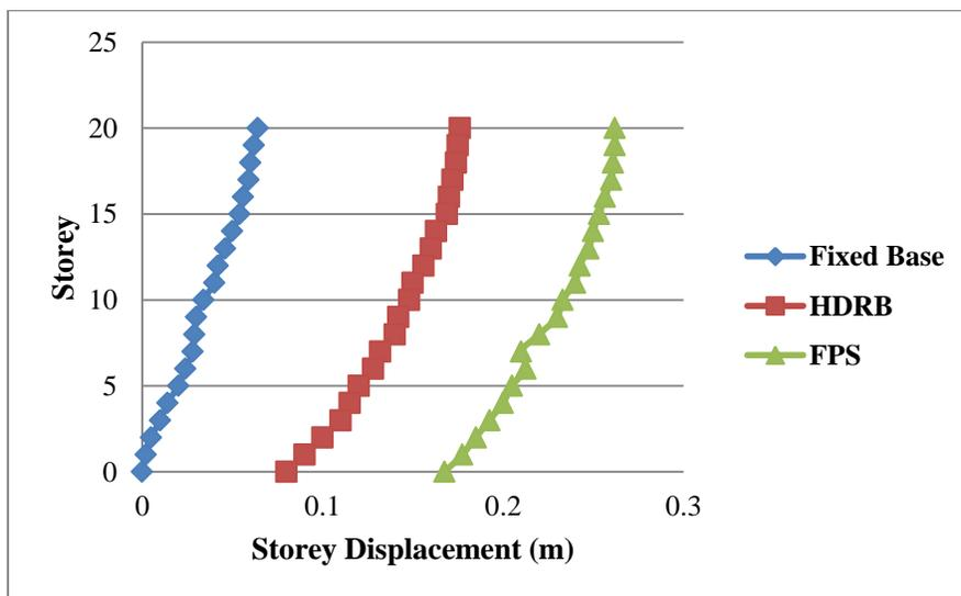
Figure 4.2.1.4 Storey Displacement in Y-Direction
