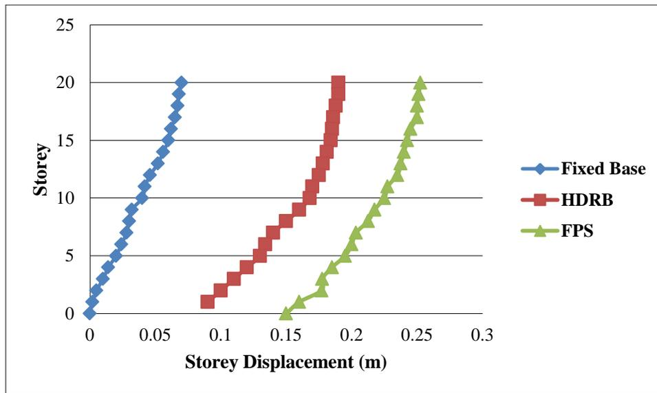
Figure 4.2.1.3: Storey Displacement in X-Direction
