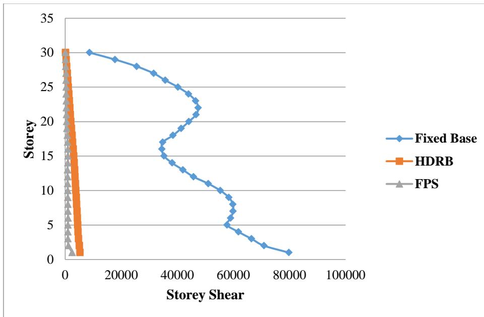
Figure 4.2.4.8: Storey Shear in Y- Direction
