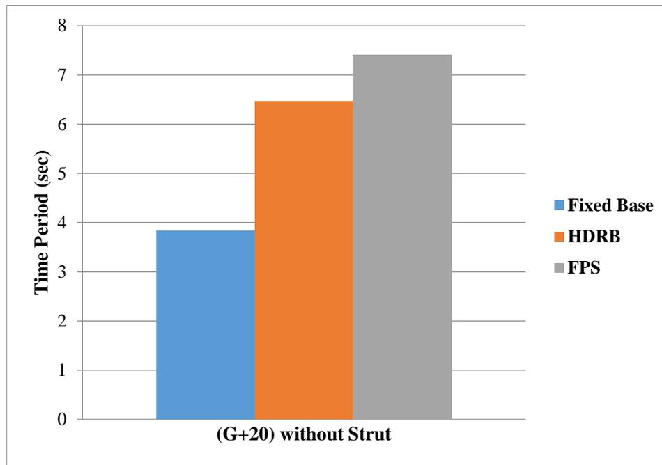
Figure 4.3.1.1: Time Period for (G+20) Storey Structure without Strut
