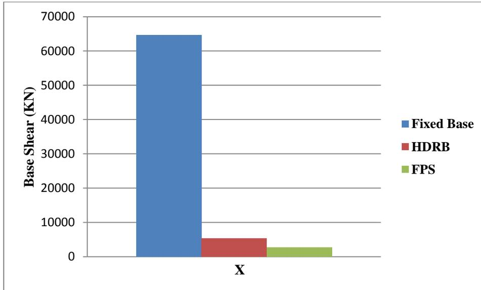
Figure 4.2.3.1 Base Shear in X-Direction
