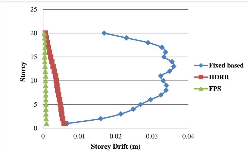
Figure 4.2.1.5: Storey Drift in X-Direction
