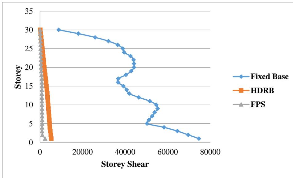
Figure 4.2.4.7: Storey Shear in X- Direction
