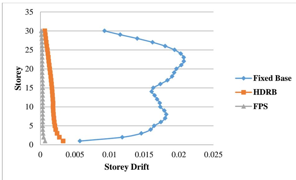
Figure 4.2.4.6: Storey Drift in Y- Direction
