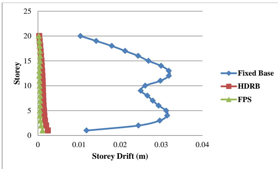
Figure 4.2.2.6: Storey Drift in Y-Direction
