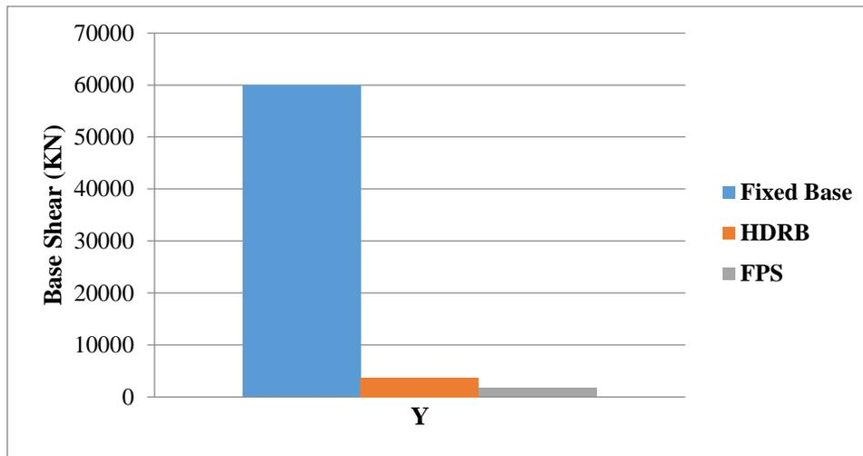
Figure 4.2.1.2: Base Shear in Y-Direction
