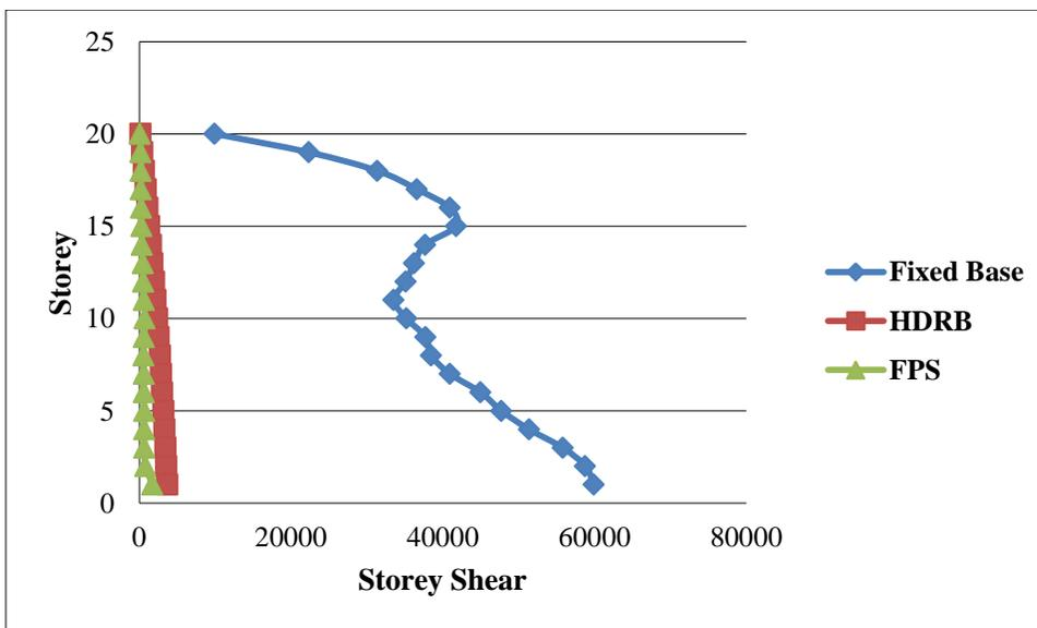
Figure 4.2.1.8: Storey Shear in Y-Direction
