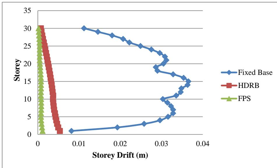
Figure 4.2.3.5: Storey Drift in X-Direction
