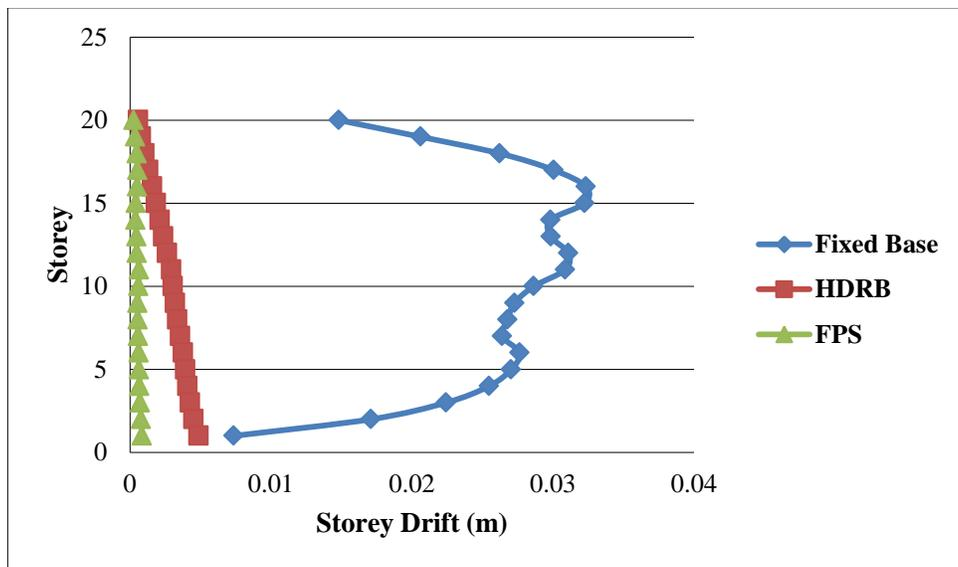
Figure 4.2.1.6: Storey Drift in Y-Direction
