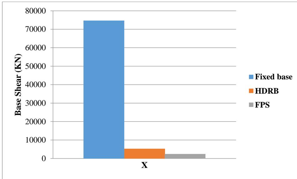
Figure 4.2.4.1: Base Shear in X Direction
