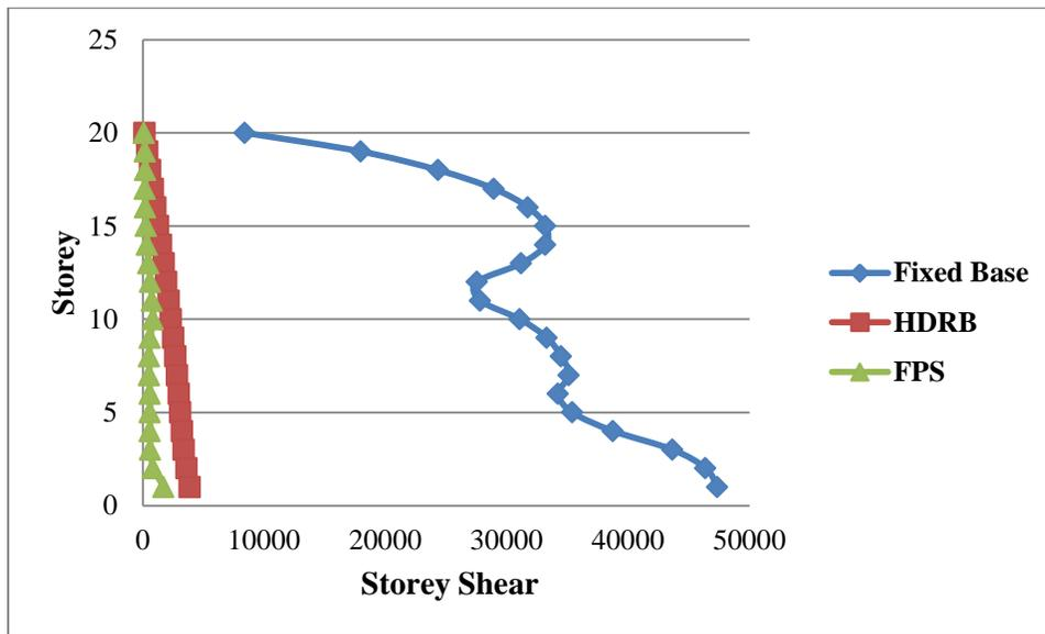
Figure 4.2.1.7: Storey Shear in X-Direction
