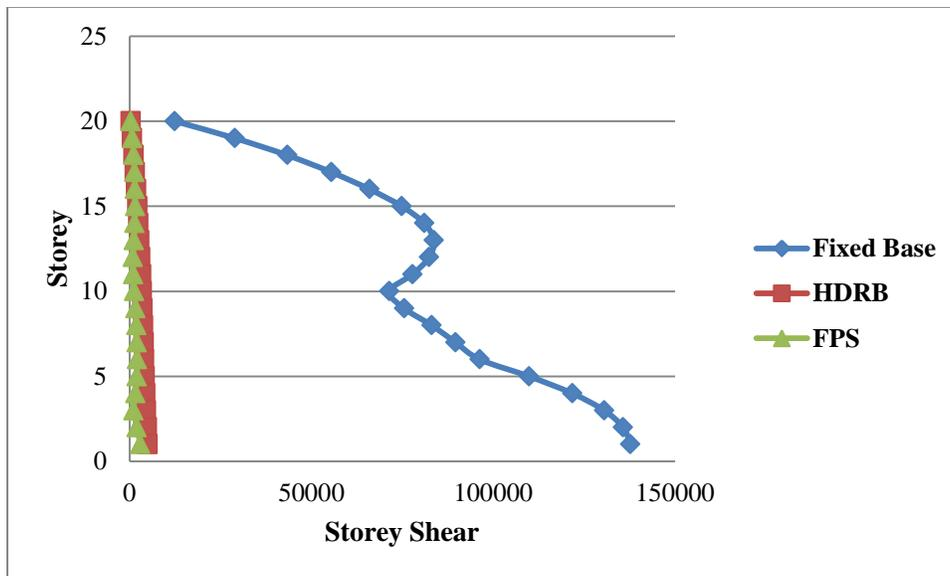
Figure 4.2.2.8: Storey Shear in Y-Direction
