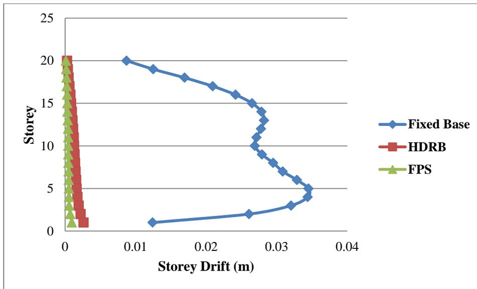
Figure: 4.2.2.5 Storey Drift in X-Direction
