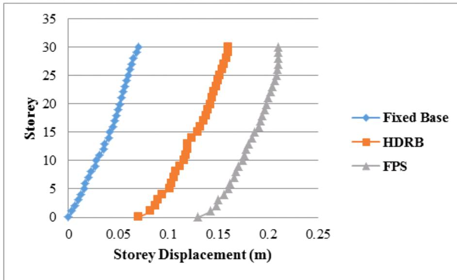
Figure 4.2.4.3: Storey Displacement in X- Direction
