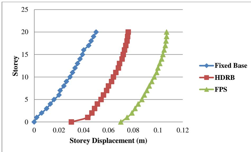
Figure 4.2.2.3: Storey Displacement in X-Direction
