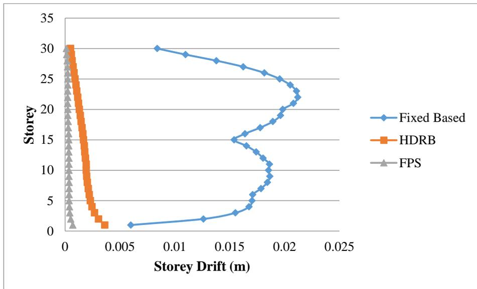
Figure 4.2.4.5: Storey Drift in X- Direction
