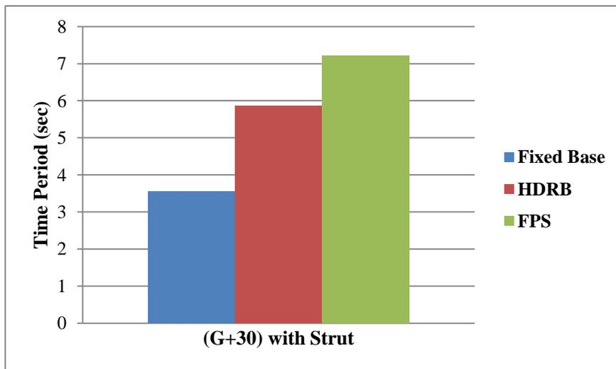
Figure 4.3.4.1: Time Period for (G+30) Storey Structure with Strut
