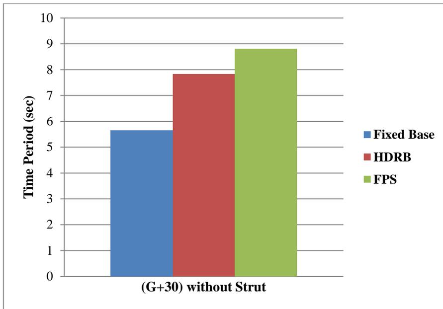
Figure 4.3.3.1: Time Period for (G+30) Storey Structure without Strut
