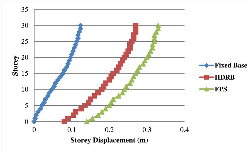
Figure 4.2.3.3: Storey Displacement in X-Direction
