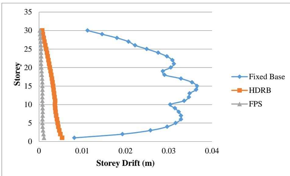
Figure 4.2.3.6: Storey Drift in Y-Direction
