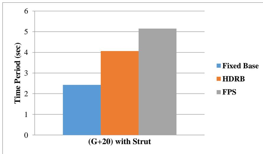
Figure 4.3.2.1: Time Period for (G+20) Storey Structure with Strut
