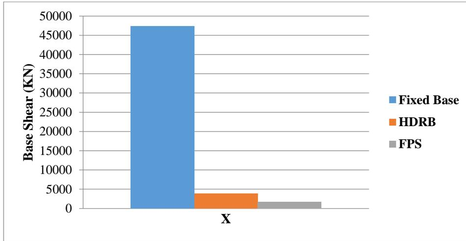
Figure 4.2.1.1: Base Shear in X-Direction
