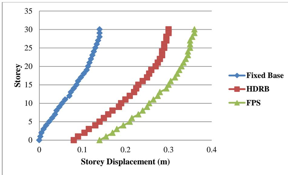
Figure 4.2.3.4: Storey Displacement in Y-Direction
