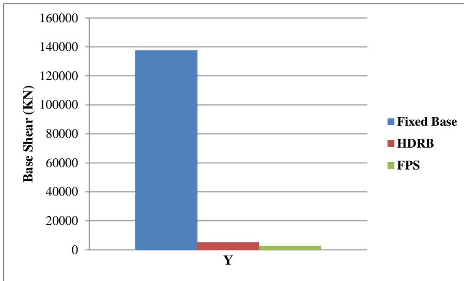
Figure 4.2.2.2: Base Shear in Y Direction
