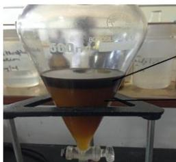
**Fig 3: Two layers formed after the acid catalyzed stage.**
