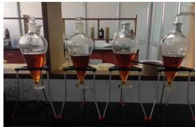
**Fig 3.4: Final methyl ester of neem oil formed after the hot water washing.**
