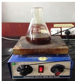
**Fig 2 Pre heating of neem oil on magnetic stirrer with hot plate.**
