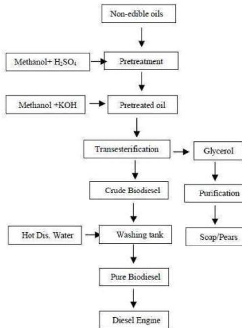
Fig 1 Process of bio diesel
