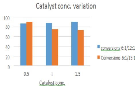
**Fig 7 variation of conversions with catalyst concentration for the 6:1 molar ratio of acid catalyzed oil for base catalyzed stage of molar ratio 12:1 and 15:1.**
