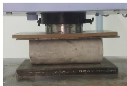
**Fig -5:** Split Tension Test on Cylinders
