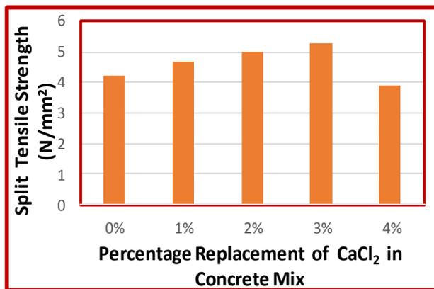
**Chart-2:** Split Tensile Strength of Cylinder Samples
