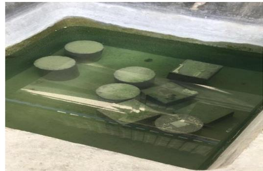
**Fig -3:** Curing of Samples
