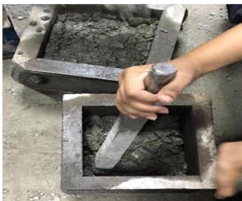
**Fig -2:** Compaction of Cube Samples
