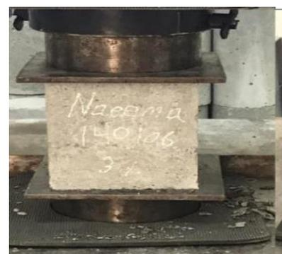
**Fig-4:** Compression Test on Cubes
