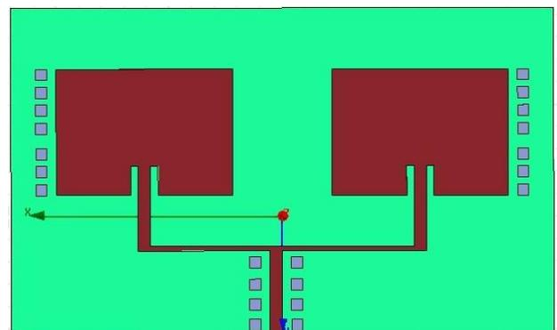
Fig 2. Simulated 2X1 microstrip patch antenna design with EBG
