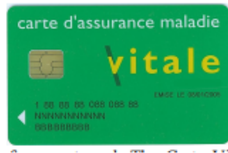
Fig-1: An example of a smart card: The Carte Vitale used for health insurance purposes in France.
