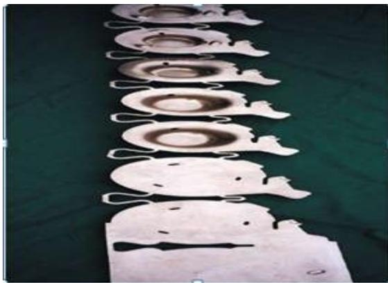
**Figure 8:** The parts shown here are carried by the scrap between them, which also serves as stretch webs for the center draw.
