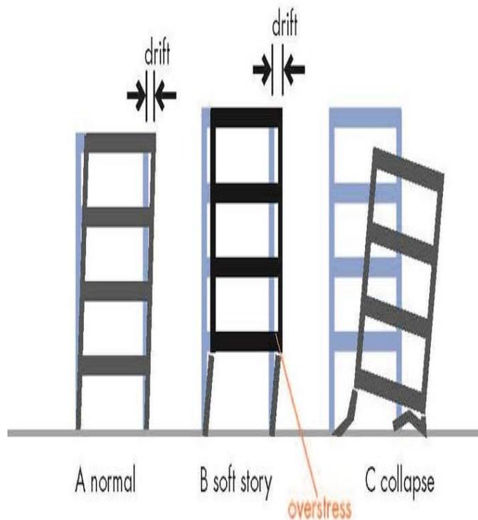
Fig -1: Soft story failure
