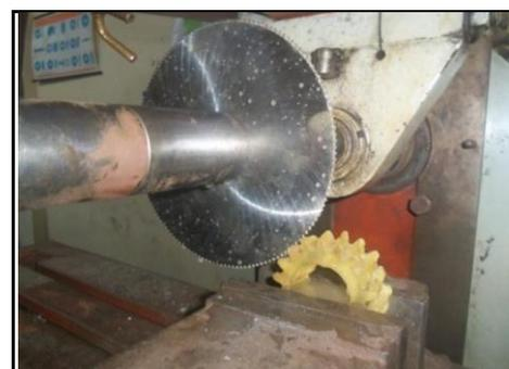
**Figure 5.3 Slicing of a stress frozen photoelastic pinion**
