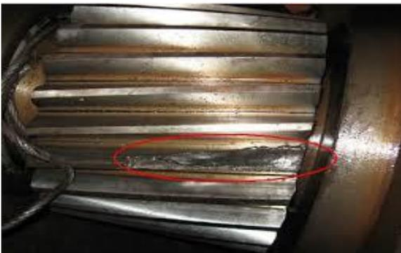
Fig .3.1 Damaged Helical Gear of Gearbox
