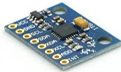
Fig.4 MPU6050 (MEMS) Micro Electromechanical System.
