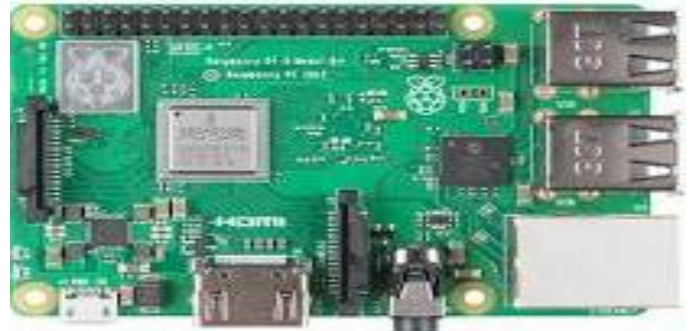
Fig. 4. Raspberry pi B 3+
