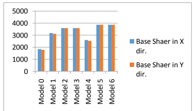
Fig. 3: Base Shear Variation in the Various Models along X-direction and Y-direction [Response Spectrum Analysis]
