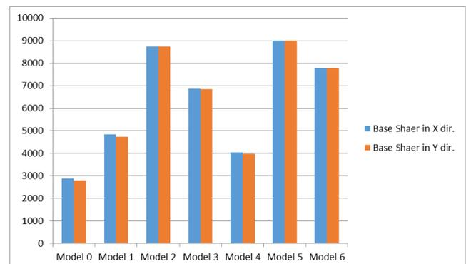
**Fig. 1:** Base Shear Values of the various Models [Equivalent Linear Static Analysis]
