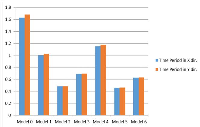
Fig. 2: Natural Time Period of Vibration of the various Models [Equivalent Linear Static Analysis]
