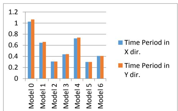
Fig. 4: Natural Time Period Variation in the Various Models along X-direction and Y-direction [Response Spectrum Analysis]
