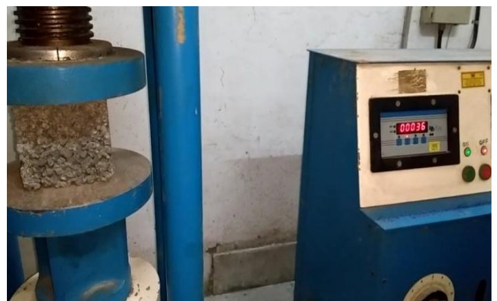
Fig 5: Compressive strength test
