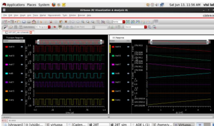
Fig: output waveform of 4-bit parallel adder using 28t
