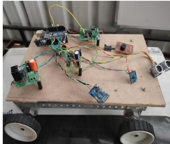
**Fig.4** Final Setup of Robot Car for demonstrating Drowsiness detection and Alcohol Intoxication
