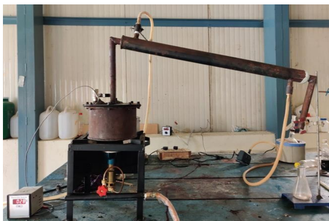
Fig -5: Experimental Setup of Pyrolytic Distillation
