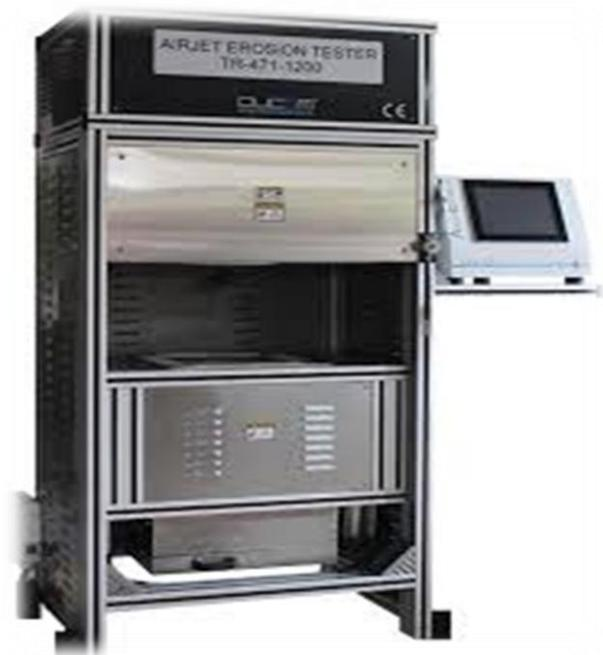
**Fig- 2:** Ducom Gas Jet Erosion Test Rig
