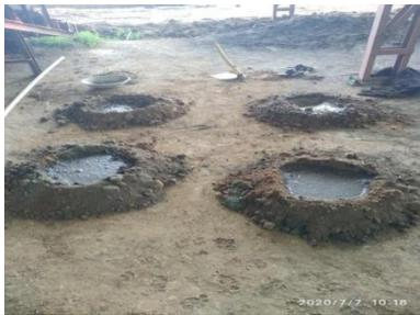
Plate 5: mixing various proportion of dry sludge and copper tailings with clay
