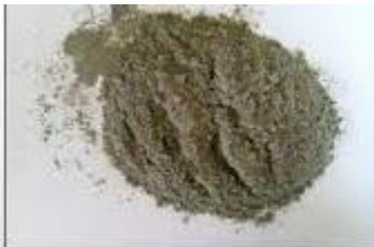
**Plate 4:** Copper Slag Waste after Pulverization
