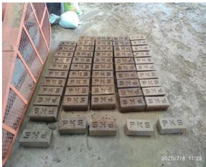
Plate 6: Various Proportion of Sludge and Copper Slag Bricks
