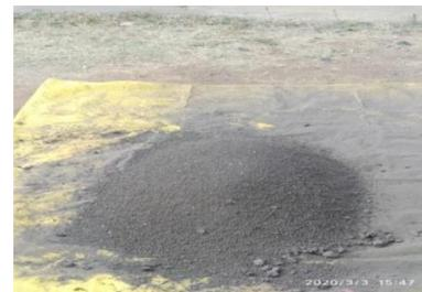
Plate 3: Crushed Dry Sludge
