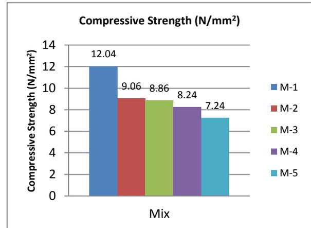
Chart 1: Graph on Compressive Strength of Produced Brick
