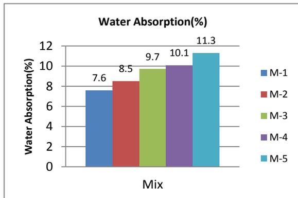
Chart 2: Graph on Water Absorption Test of normal and Produced Bricks.
