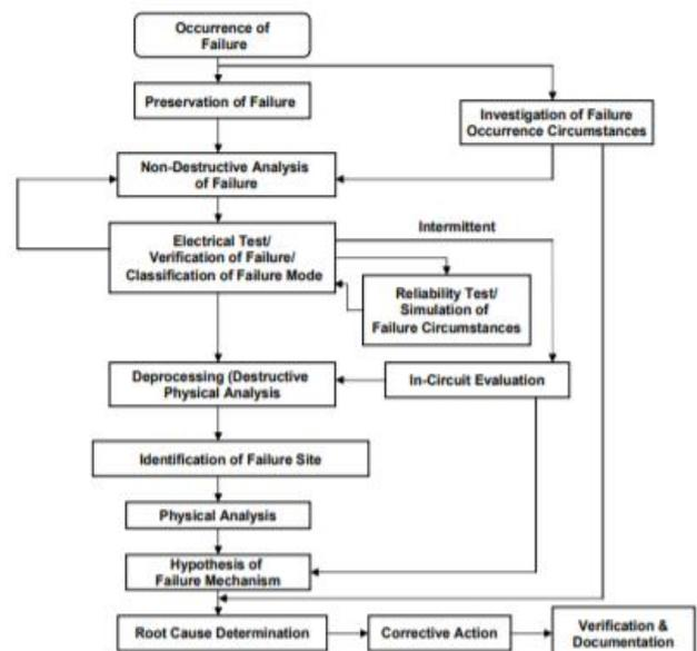
**Fig -2:** FA Process Flow of Electronics
