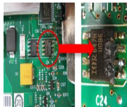
Fig -7 Burned component
