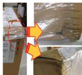
Fig-4 Crushed Packaging
