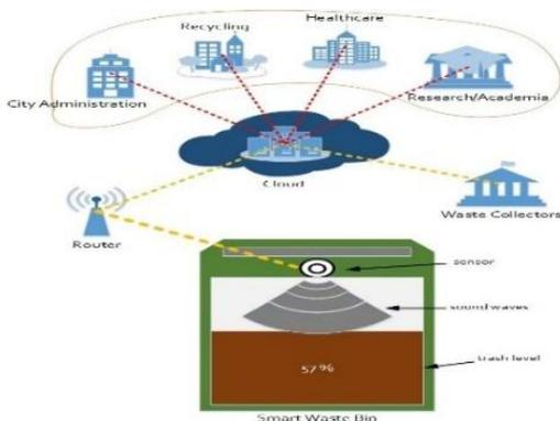
Fig 1: Cloud based SWM Architecture
