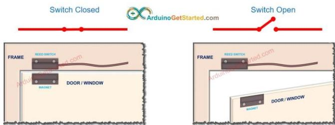
If we connect a pin of the reed switch to **GND**, the other pin of the reed switch to Arduino's input pin with a pull-up resistor (internal or external):
