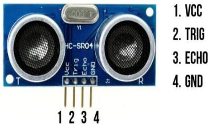
In order to generate the ultrasound, we need to set the **Trigger Pin** on a **High State** for **10 μs**. That will send out an 8 cycle sonic burst which will travel at the speed of sound and it will be received in the Echo Pin. The Echo Pin will **output the time** in microseconds the sound wave travelled.
