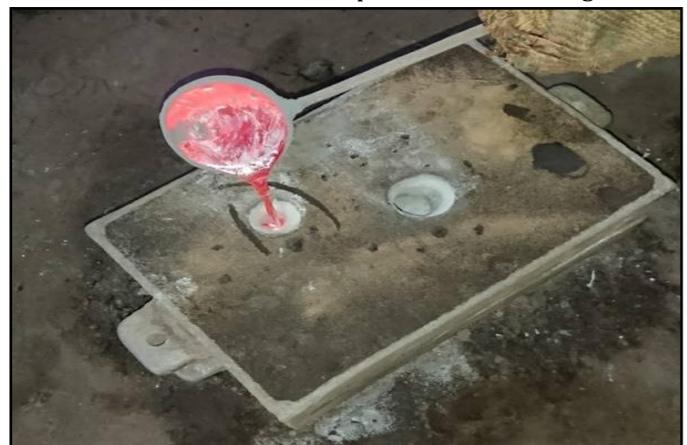
**Fig -1:** Pouring of Molten metal
