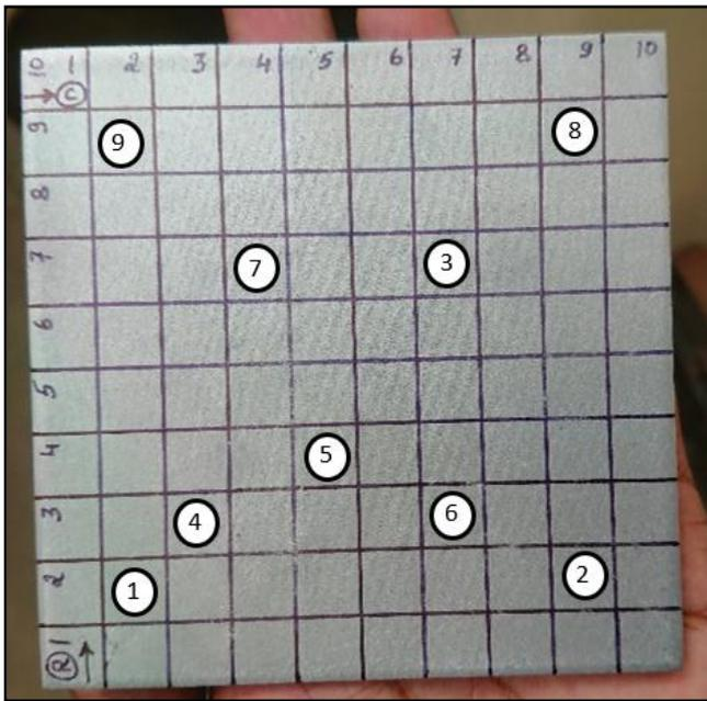
Fig-8: Random places where Hardness is measured
