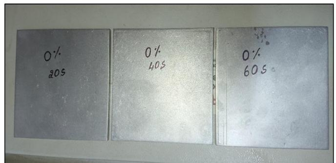
Fig-7: Plates subjected to multiple shocks
