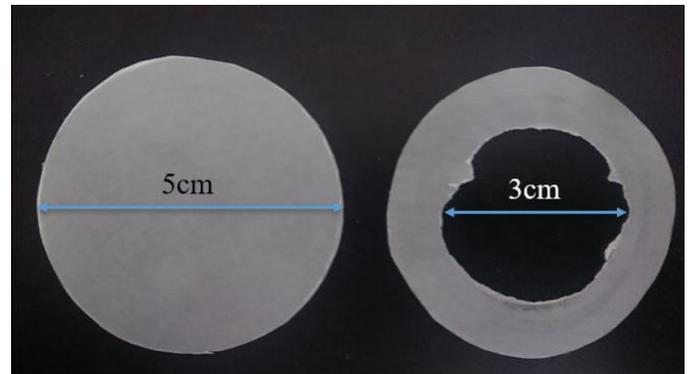
Fig-6: Diaphragm before and after it ruptures
