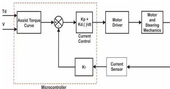
Fig. 2 Schematic Diagram of a Model EPS Control Unit
