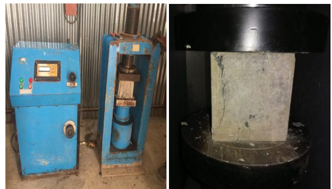
Photos of doing compressive strength test.
