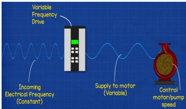
Figure-1: Variable frequency drive
