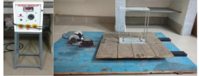
Figure 3.1: RPM controller of D.C. motor and Shake table setup
