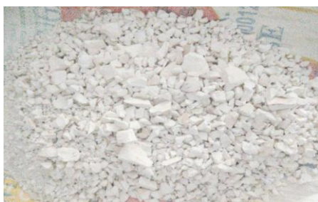
Fig.01: Dry paint waste
