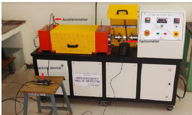
Fig -5: Experimental Setup of Gearbox Test Rig
