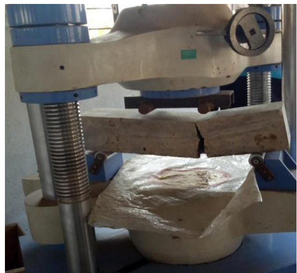
Fig -2: Flexural strength testing
