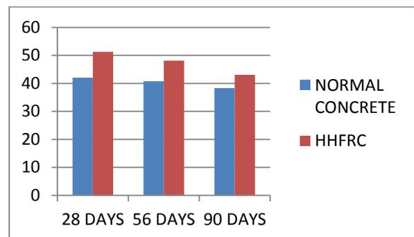
**Figure- 5 Compressive Strength of Concrete Cubes in Sea Water**
