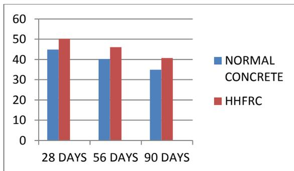
**Figure- 3 Compressive Strength of Concrete Cubes in H<sub>2</sub>SO<sub>4</sub> Solution**
