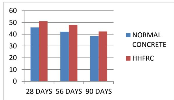
**Figure- 4 Compressive Strength of Concrete Cubes in MgSO<sub>4</sub> Solution**
