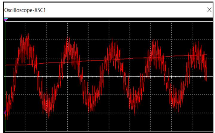
**Figure-4** Dynamic response of Electromagnetic Torque(per Nm/μsec) For 12 poles.
