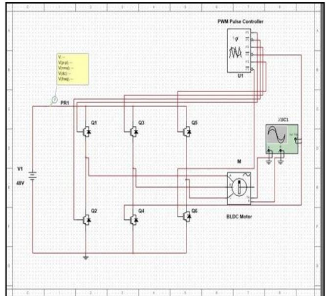
Figure-2 Simulation Circuit for Module
