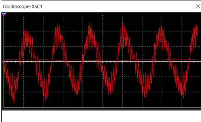
**Figure-3** Dynamic response of Electromagnetic Torque(per Nm/μsec) For 6 poles
