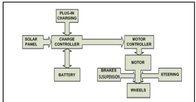
Figure -1: Block Diagram of Solar Module Electric vehicle
