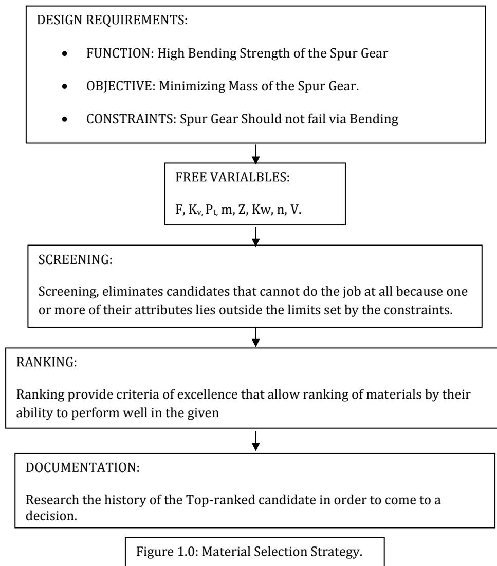
The Material Index is found out after a careful evaluation of the constraints, objectives, function and free variables (the material index is evaluated in the later part of this study). The Performance of the structural element is determined by three things as per Ashby Method: The function Requirement, The Geometry and the properties of the material of which it is made [6]. It is best Described by the following equation:
