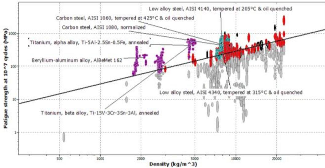
Figure 7.0: Strength Vs. Density Graph only for metals
