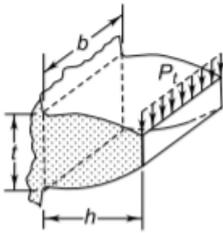
Figure 2.0: Gear tooth as a Cantilever Beam
