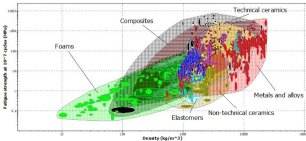
Figure 5.0: Material Families in Fatigue Strength Vs. Density.
