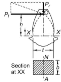
Figure 3.0: Gear tooth as parabolic beam
