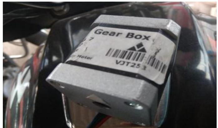
Fig -4: DC Stepper Motor
