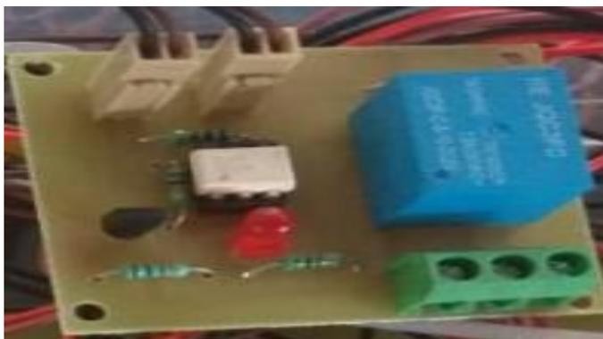
Fig -3: Relay Circuits
