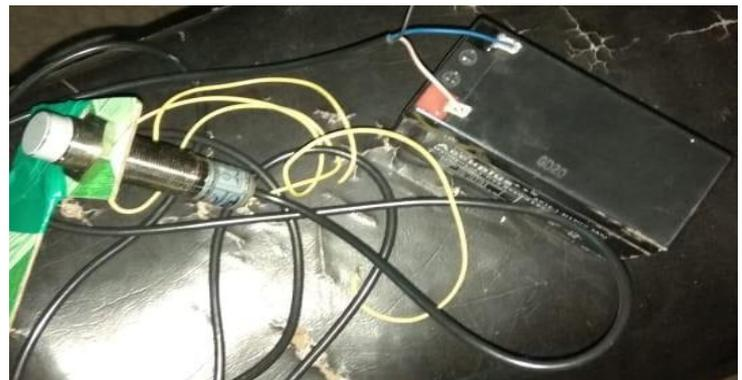
Fig -1: Proximity sensor connected with battery
