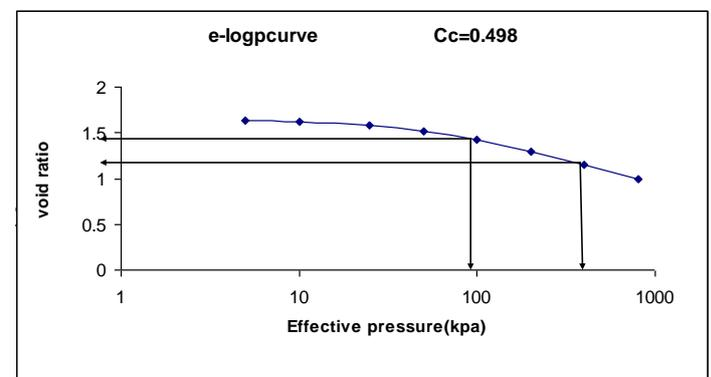
Fig 4.1 Plot for log of effective pressure v/s void ratio.
