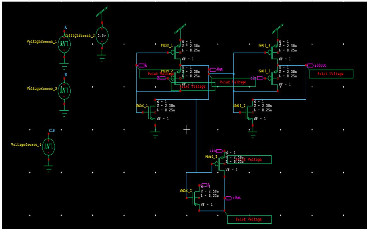
**Figure 2:** Full adder design implementation by using transistor and xnor gate
