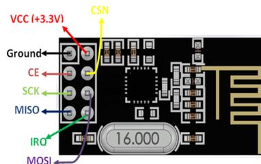
Figure 2: NRF24L01 Module
