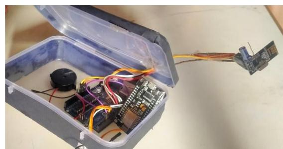
Figure 4: Receiver node / Gateway node
