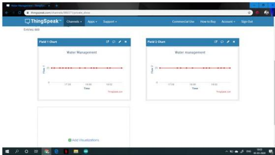
Figure 5: flow meter graph when No leakage occurs
