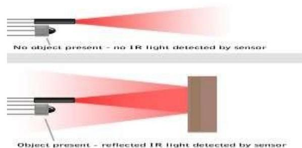
Fig-3: IR Sensor operational diagram
