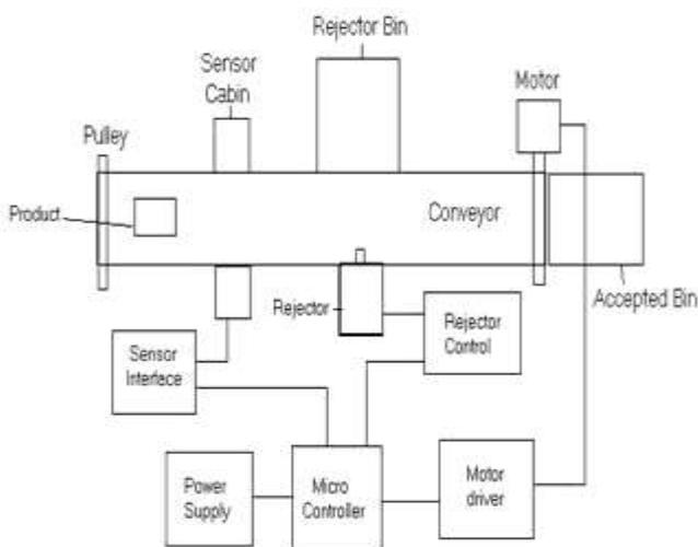
Fig-5: CONCEPTUAL DIAGRAM
