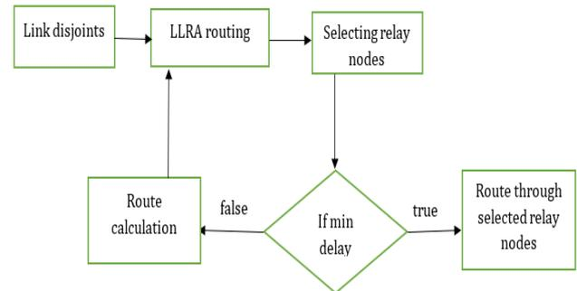
Fig-4: Low Latency Routing Algorithm (LLRA)
