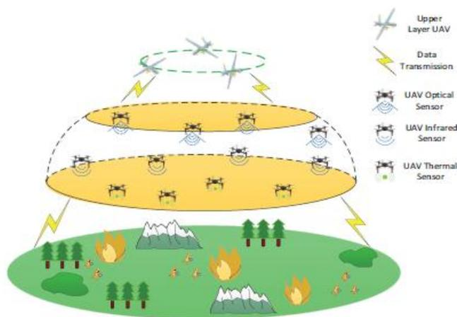
Fig-1: Typical Layered UAV Network
