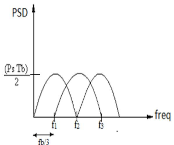
Figure 2- Bandwidth with spectral overlap [1-2]
