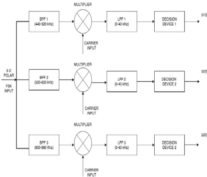
Figure 3- 3-Dimensional polar FSK Receiver
