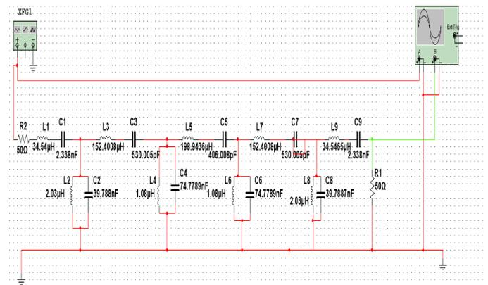
Figure 6- Bandpass filter 2 design
