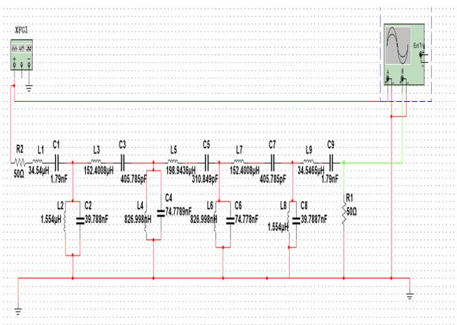
Figure 8- Bandpass filter 3 design
