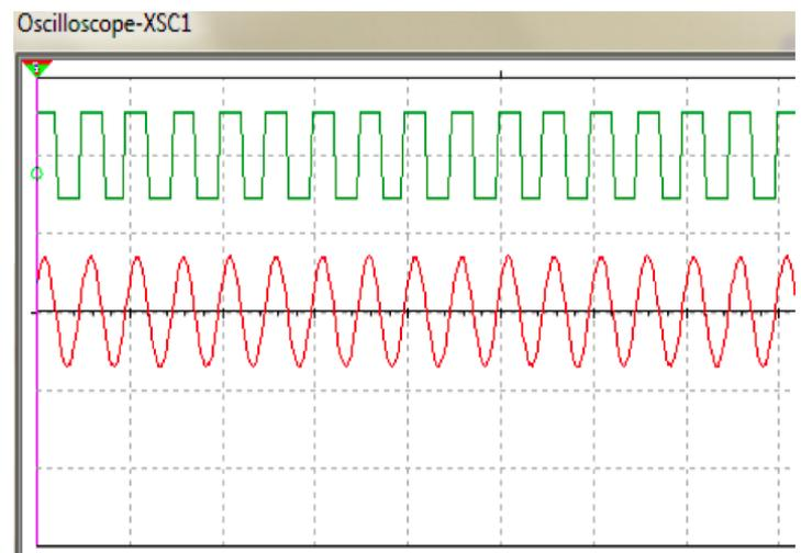
Figure 14- Comparator simulation output
