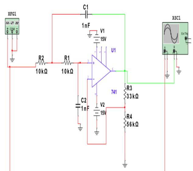
Figure 11- Low pass filter design
