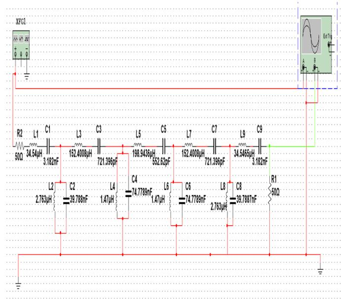
Figure 4- Bandpass filter 1 design
