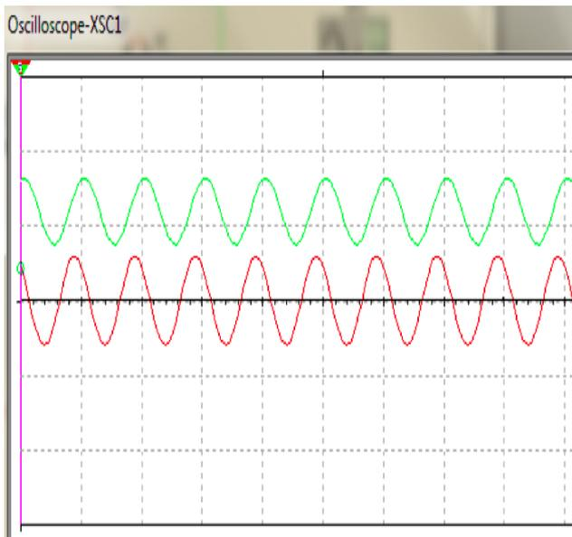
Figure 12 -Low pass filter simulation output
