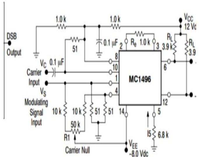
Figure 10 - Multiplier circuit diagram
