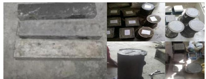
Figure 1: Casting of Cubes, Cylinders and Beams
