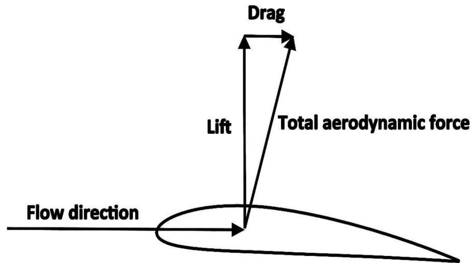
Figure 1. Airfoil Aerodynamic forces.
