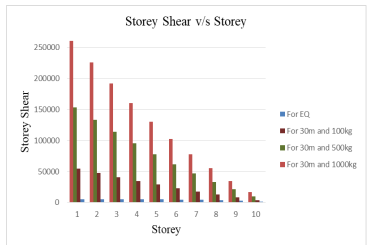
Fig .3.4: Storey Shear of the building for Seismic analysis and also for various cases of blast.
