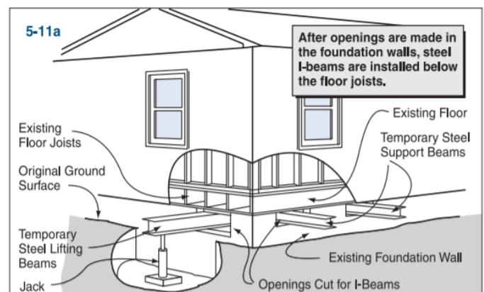
Fig. 5. Cutting holes and inserting I-Beams in foundation walls.
