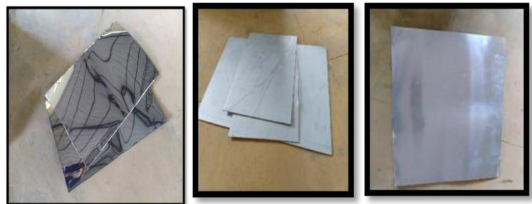
Fig -2: Straight sheet pile made of stain less steel(left) and GI sheet (Centre) Aluminium sheet pile(right)
