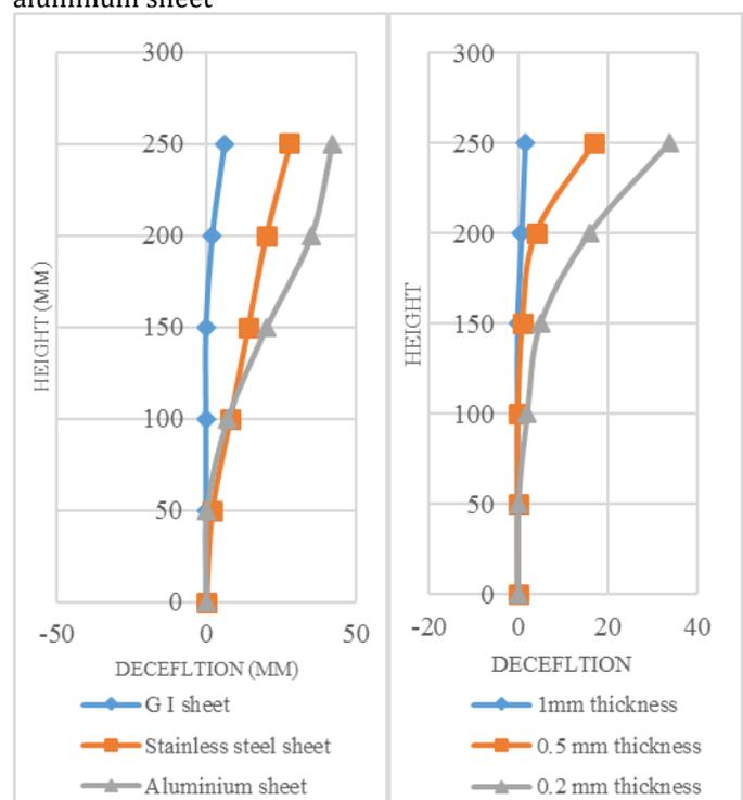
Chart -1: Height - deflection graph when different material (left) used and different thickness used (right)
