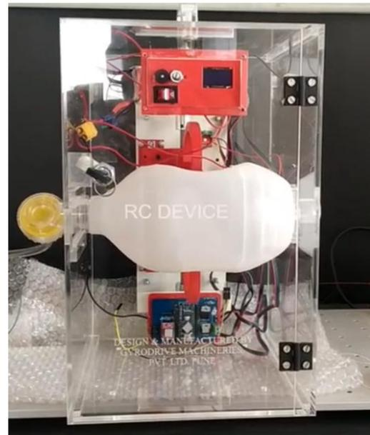
**Fig 9:** Prototype of Low Cost Respiration Control Device
