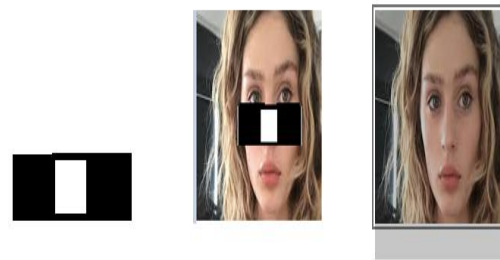
HAAR Feature which are similar to each other forms the bridge of the nose
